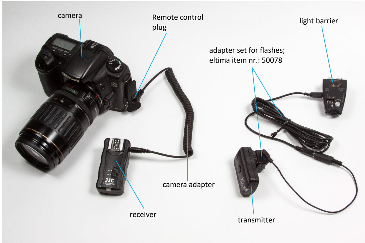
Figure 1: Connecting a camera via radio remote control
