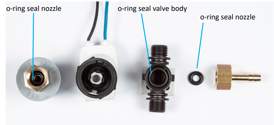
Figure 17: solenoid valve disassembled
