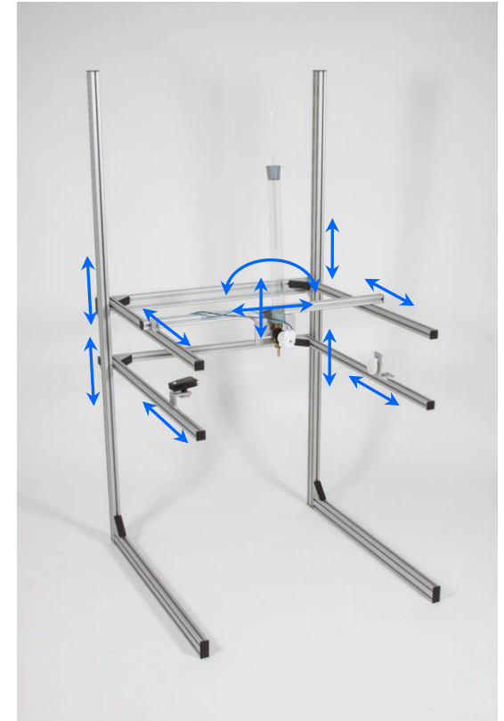
Figure 23: adjustment options of the carrier system
