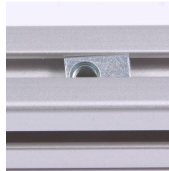
Figure 2: inserting the second edge of the nut into the slot
